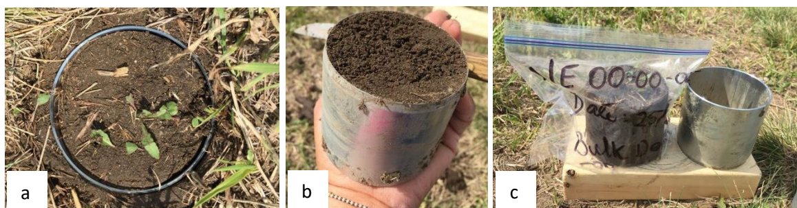
Picture 10. Soil core ring 3 by 3 inches soil surface (a), whole core (b), BD soil in sealable labeled bag (c).
