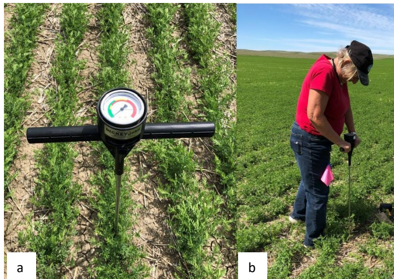
Picture 9.- a) Soil Compaction Meter: Penetrometer, b) Penetrometer measurement
