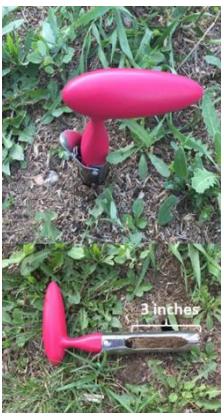
Picture 1. Apple corer 1" diameter, 3" depth
