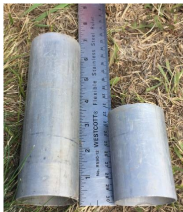
Picture 2. 2" Diameter rings: 3 and 6" depth
