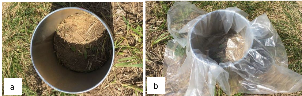
Picture 6.- a) Ring pushed 2 inches deep, b) plastic wrap lining inside the ring
